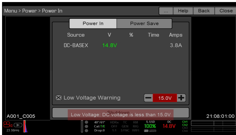
Figure: Low Voltage Warning
